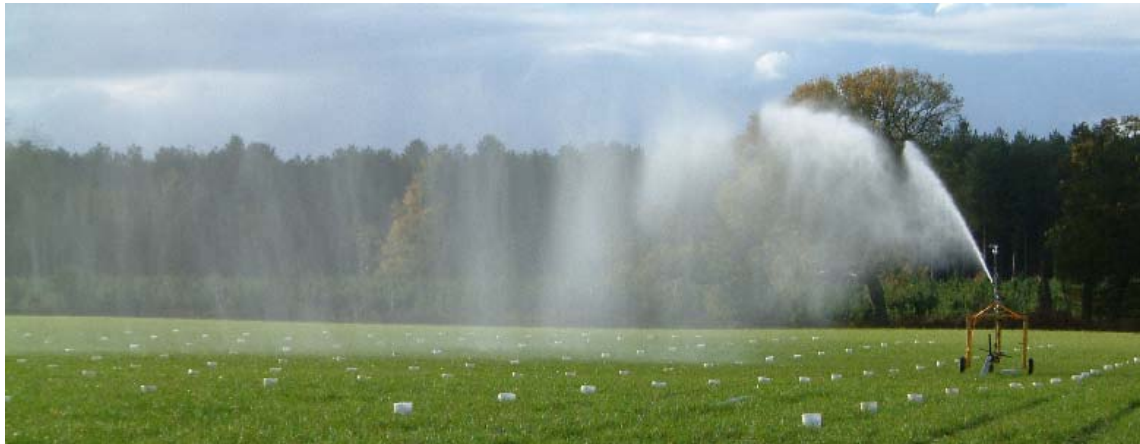
Figure 4.13 Wetted pattern measurement at site R2004 under a wind speed of approximately 3.7 \text{ m s}^{-1} .
